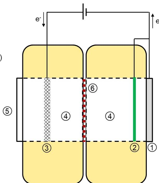
Top left and right: schematic of the electrochemical cell used for HP production.
