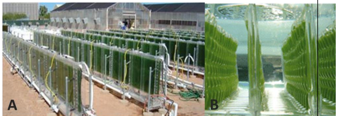
Figure 1 Conventional flat panels (A) and submerged flat panels (B) designs similar to the ones considered in the techno-economic analysis.
